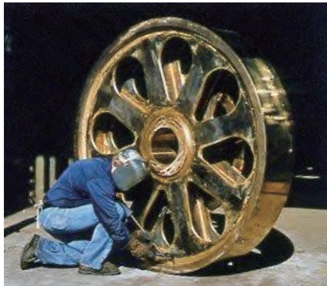
Propulsor Gear: Aluminum Bronze cast & wrought components fabricated into a 4000 lb. propulsor gear for a minesweeper.
