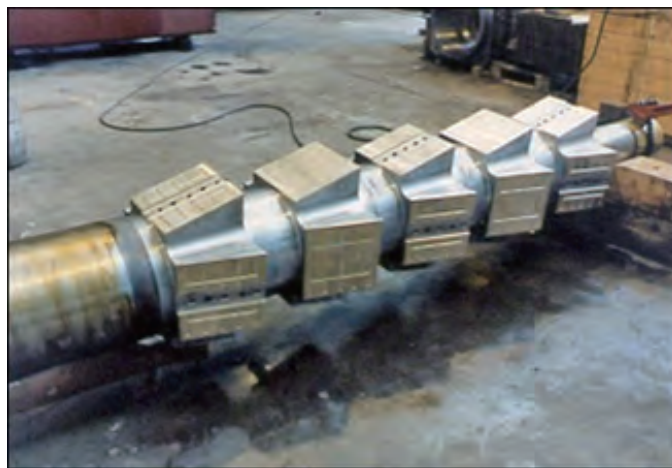
Main support shaft of steel mill coiling machine AMPCO-faced to resist abrasion and wear.
