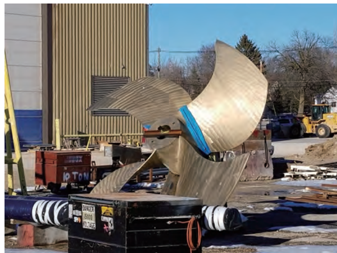
Superston ship propeller repair welded with AMPCO-TRODE® 40.
