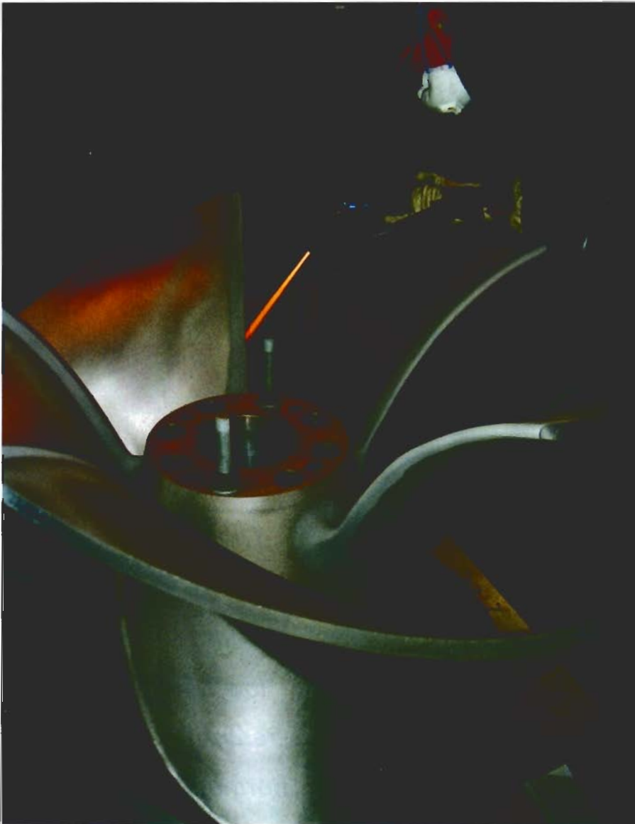
Fig. 2 — The leading edges of this impeller receive a wear-resistant carbide coating using the HVOF thermal spray process.
